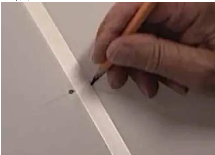
Figure 24. A premarked location for a lacing hole, which is punched through the fabric with a pencil.
