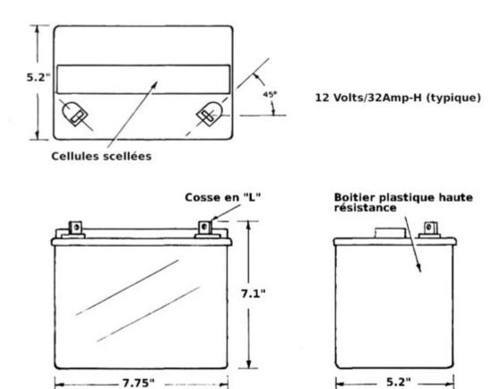
Batterie avion cellules gel (dimensions types)
