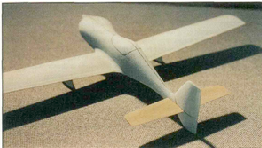
AR-6 showing high pressure area on horizontal stabilizer (left half of airfoil) meeting low pressure area on vertical stabilizer (around point of maximum thickness on vert. stab.).
