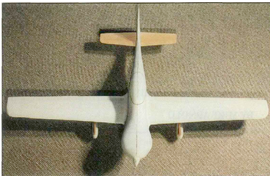
AR-5 Formula 1 design, showing engine cowl fairing in to fuselage sides over point of max. thickness on wing. Fuselage sides are then parallel back to trailing edge.
