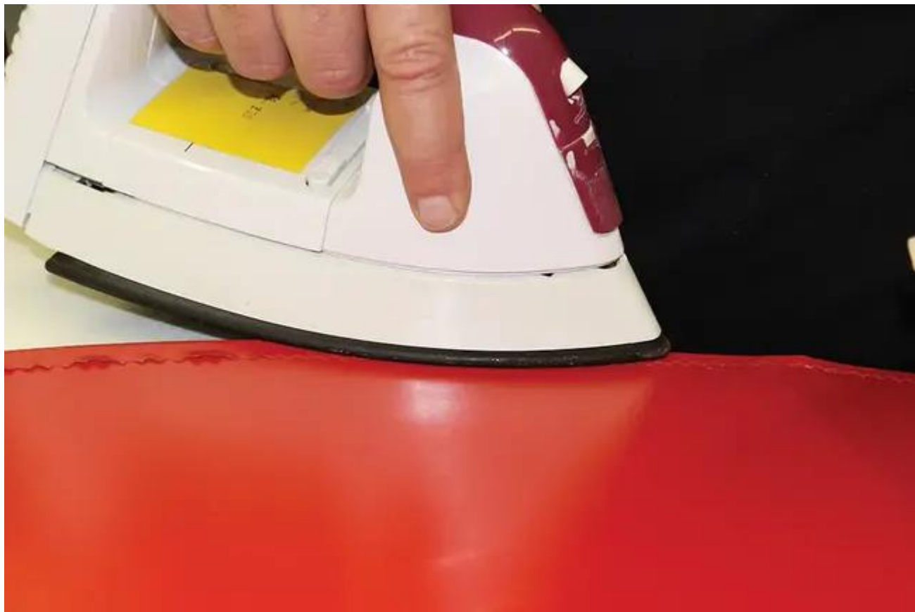
Fig. 9: When heat is applied to the center of the tape, it stretches enough to allow the non-heated, and now shorter, edges to lie down. They can be smoothed with an iron.
